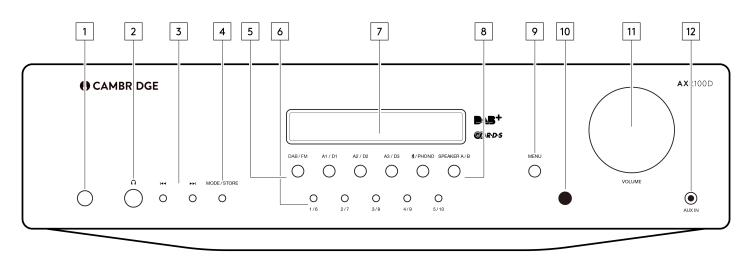
**1. POWER BUTTON** - Switches the unit between Standby mode (indicated by dim power LED) and On (indicated by bright power LED). Standby is a low power mode where the power consumption is less than 0.5 Watts. The unit can be left in Standby mode when not in use.
